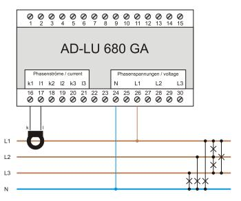
3 Phasen, 3 Leiter, ungleiche Last 3 phases, 3 wire, unbalanced load
