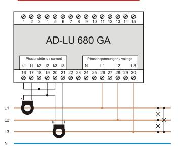
3 Phasen, 3 Leiter, gleiche Last 3 phases, 3 wire, balanced load
